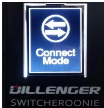
2. Carefully disconnect the display (green) plug on your electric bike and connect the Switcheroonie into the plug on your bike; once secure, press the tick button to connect.
