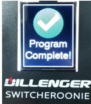
9. Once uploaded successfully, unplug the Switcheroonie and plug your display back in to complete the change.
